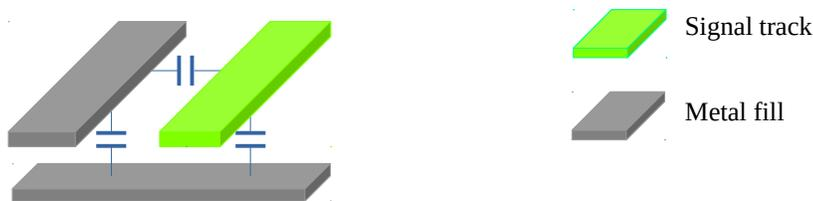
Figure 1: Signal track-metal fill coupling
