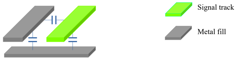
Figure 1: Signal track-metal fill coupling
